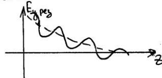
$$\delta) \omega_{kp20} = \lambda_{20} \cdot c = \frac{2\pi c}{a} \Rightarrow f_{kp} = \frac{c}{a} = 3000 \text{ МГц.} \Rightarrow \text{TE}_{20} - \text{нераспр. мода}$$
