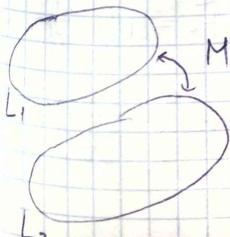
$$\begin{aligned} W_u &= \frac{L_1 I_1^2}{2} + \frac{L_2 I_2^2}{2} + MI_1 I_2 = \\ &= \frac{1}{2} (L_1 I_1^2 + L_2 I_2^2 + MI_1 I_2 + MI_2 I_1) = \\ &= \frac{1}{2} I_1 (\underbrace{L_1 I_1 + M I_2}_{\Phi_1^{\text{нек}}}) + \frac{1}{2} I_2 (\underbrace{L_2 I_2 + M I_1}_{\Phi_2^{\text{нек}}}) \end{aligned}$$
